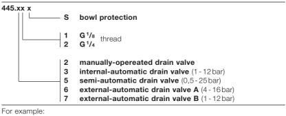
445.22 – but with semi-automatic drain valve and bowl protection = 445.52  $\underline{S}$
