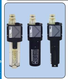
Lubricators add a fine oil fog to the compressed air, this effecting a constant and reliable lubrication of pneumatically controlled compressed air tools, valves and cylinders etc... Refilling oil while under pressure is possible. Needle valve for oil adjustment with high drop constancy for long periods of time. Also available with metal sight dome.
