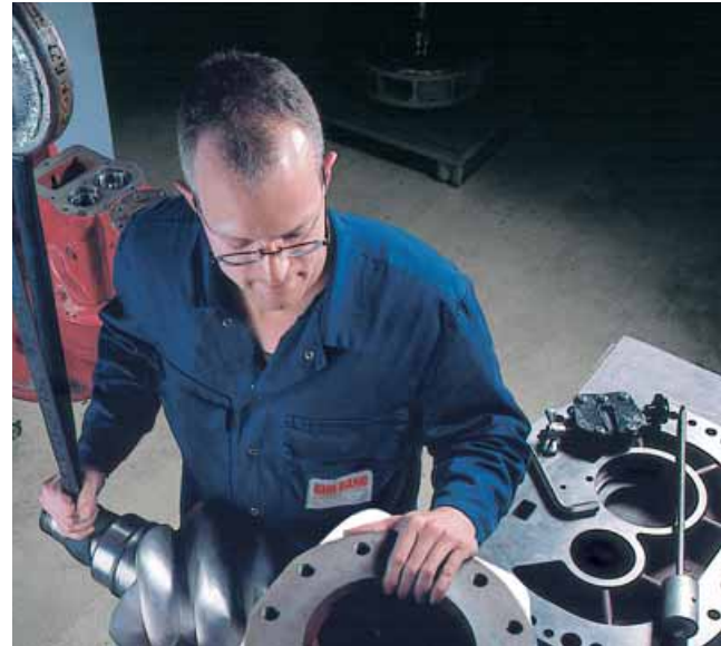
A GHH RAND service technician inserts the male rotor within the rebuild of a CF180G.
